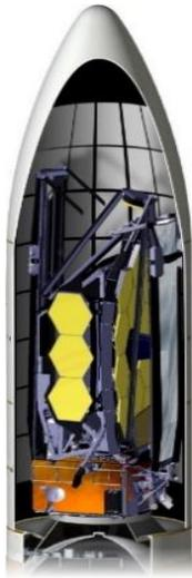
Figure 3 JWST Observatory Launch Configuration (Masetti, *About Webb Launch*, 2019)
