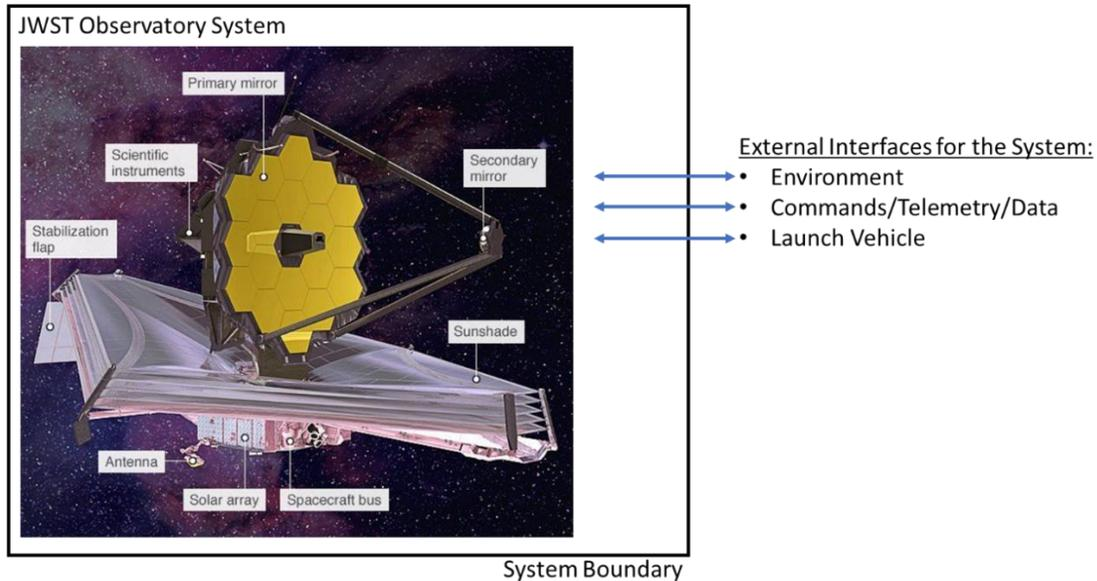
Figure 2 Architecture Diagram of the Observatory Segment (Nichols, 2018)
